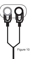
Typical speaker output using spade connectors. Insert bare wire into the binding post and tighten. **SPEAKON ASSEMBLY:** You will need a pair of Neutrik Speakon® NL4FC connectors. You will also need high-quality two or four conductor speaker cable, a pair of needle-nosed pliers and a 1.5-mm Allen key to assemble the Speakon connectors to your speaker wire. To assemble the Neutrik Speakon NL4FC connector, complete the following steps:
